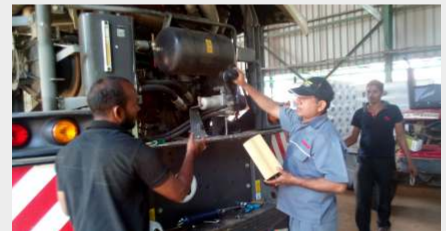
On site JAGUAR 850 schedule service of 1000 hour successfully completed using CLAAS Diagnostic system (CDS) software.
