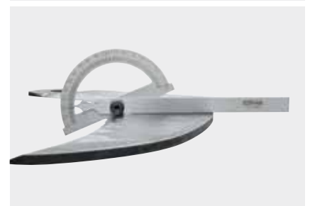
Incorrectly sharpened knife: angle approx. 22°.
