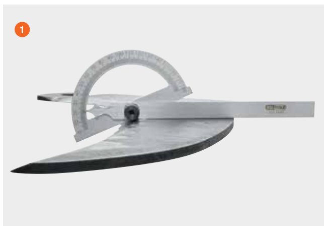
Knife with the wrong grinding angle (22°), sharpened with a manual grinding unit.
