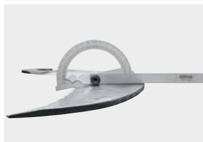
Properly sharpened knife: angle approx. 10°.
