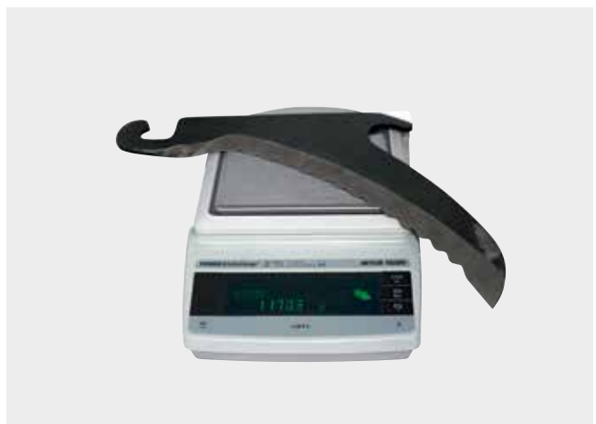
Knife sharpened to the max. abrasion limit: 1.1 kg.
