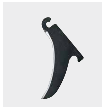
Incorrectly sharpened knife: less defined scallop pattern.
